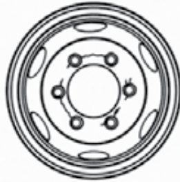
Bolt hole to bolt hole. Causes: Loose cap nuts, small hub backup (also see bolt hole cracks/distortions).
